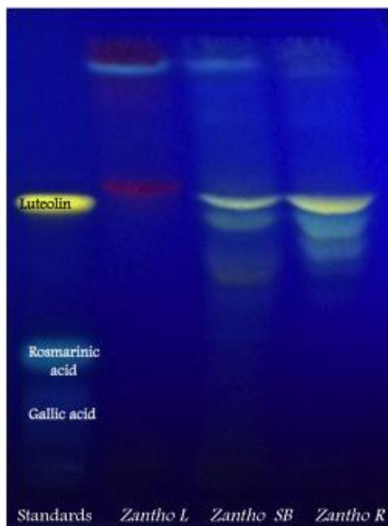
**Figure 2** TLC chromatogram of methanolic extracts from parts of *Z. gillettii* (Leaves: Zantho L, Stem bark: Zantho SB and Root bark: Zantho R) with gallic acid, rosmarinic acid and luteolin as standards; developed with dichloromethane/acetone/formic acid (85:20:10; v/v/v) and visualized at 365 nm with Natural Products-PEG reagent. Flavonoids are detected as yellow fluorescent spots and phenolic acids as blue fluorescent spots
